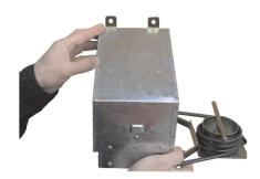
NOTE: When demonstrating or test firing the trap always use a *Soft Substrate* such as a rolled up newspaper to fire the spring. *Never* use a hard substrate like a stick. This will damage the trap.
